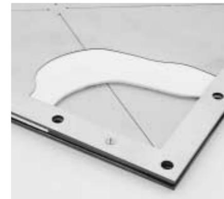
Depending on the application, the heat shield may be a thin layer of ceramic paper or a thicker layer of ceramic fibres fitted to the process side of the panel. In extreme cases heat shields can protect panels from temperatures as high as  $1000^{\circ}\text{C}$  ( $1832^{\circ}\text{F}$ ).
