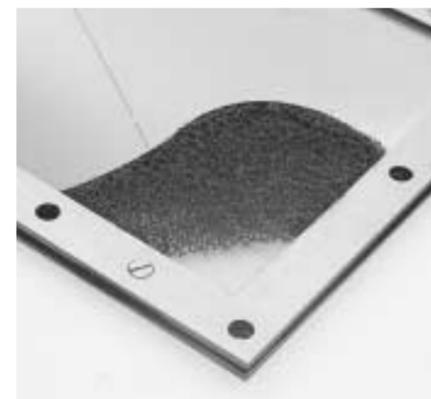
In many installations, particularly filters, the system is subjected to short, sharp pressure pulses. Though often small, these pressure pulses create a change in system pressure such that the membrane fluctuates. Where this fluctuation is frequent, as is the case with reverse jet filters, it can lead to fatigue of the slotted membrane ligaments. To overcome this, the vent side slotted membrane is domed and a foam 'damper' is fitted between the membranes to prevent any unwanted movement.
